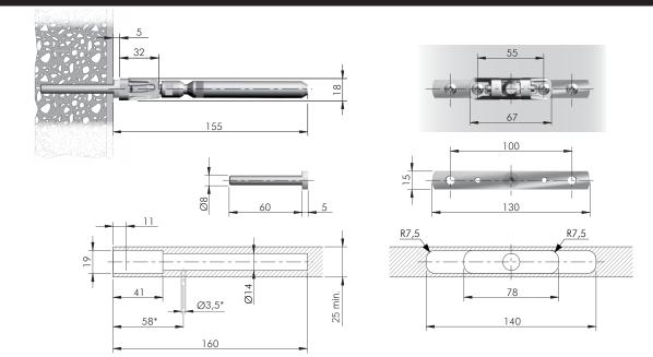
\* Optional drilling for security locking with M4 grub screw placed underneath in alignment with the cavity. For details refer to Triade Mini section.
