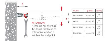
SCREW THE LOCKING BOLT TO BLOCK THE PIN
