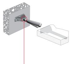
ALIGN BRACKETS VERTICALLY ACCORDINGLY
