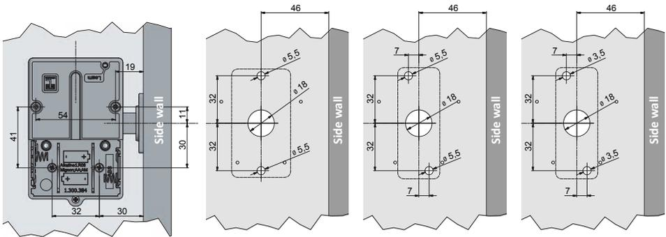
**CAUTION:** - For mounting the RFID reader L033-A02 • **without** spacer please use drill holes of 5,5mm.
