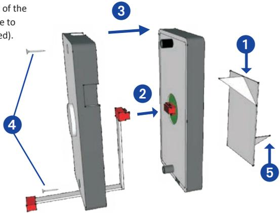
Then stick the entire reading unit to the inner side of the door.
