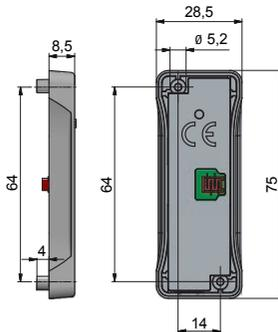
RFID reader L033-A02 with optional spacer
