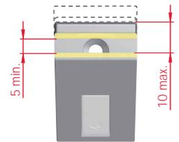
Shelf is clamped between a layer of white soft rubber on both the lower and upper side (coloured parts).
