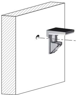
Recommended fixing countersunk screw type - head Ø 5 mm max.
