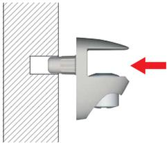
Assembling with alternative fixing options to achieve horizontal connection
