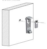
Recommended fixing countersunk screw type - head  $\varnothing$  4 mm max.
