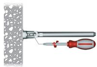
SHELF INSERTING AND LATERAL ADJUSTMENT
