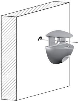
Recommended fixing countersunk screw type - head Ø 5 mm max.
