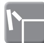
**AeroSplit** is the perfect solution for narrow kitchen or low ceiling furniture applications. The folding door is opening at an angle of 125°, ensuring that the second half of the door folds extremely flat and ensuring full accessibility of the space. The technical appeal of this product fits well with modern front design.
